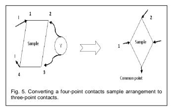
In this arrangement, there will be 6 measurements instead of 8, with three geometric factors  $f_{A_1}$ ,  $f_B$  and  $f_C$ .  $V_2$ ,  $V_4$  and  $V_6$  are measured as shown in the figure with  $V_1$ ,  $V_3$  and  $V_5$  are measured with the corresponding currents injected in opposite direction. Van der Pauw equations will be modified as follows:
