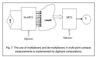
As an example, 1-8 de-MUX is used with 3 selectors to direct the sourced current to one of the 8 point contacts, and the voltage at any other point contact is selected with a *normaly* 8-1 MUX and 3 selectors.
